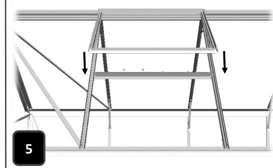
\* TIP: For aluminium finish models due to binding, a little lubricant may be needed to ease fitting of vent / windows \*
