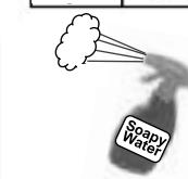
\*TIP: Spray either side of glass panes with soapy water to ease fitting of the capping\*
