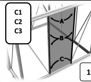
\*TIP: Spray either side of glass panes with soapy water to ease fitting of the capping\*
