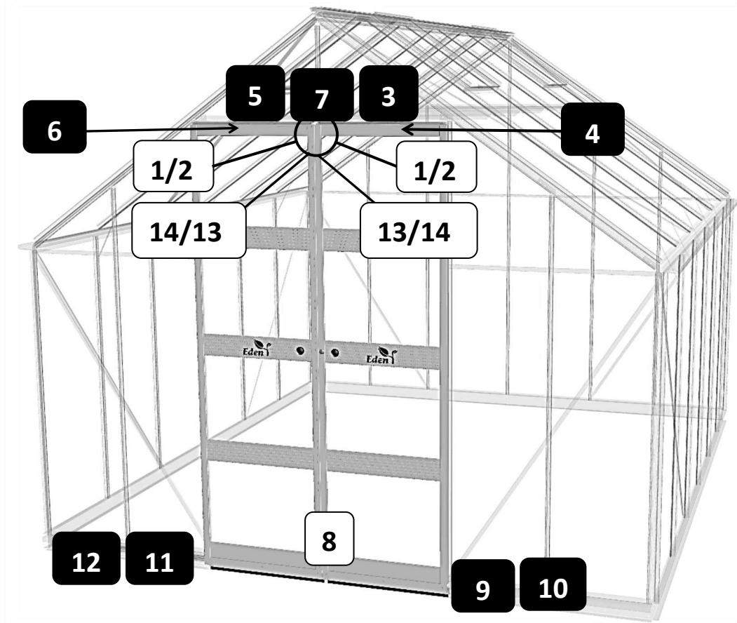
*\*TIP: Before fitting doors, please make sure the base and door aperture are level and square to ensure doors run smoothly\**
