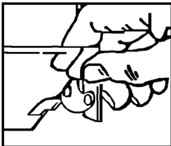
5. Finally you mount the glass you removed from the section. We recommend that you remove all silicone from the profiles before you mount the glass again. Perhaps it is necessary to adjust one piece of glass depending on which greenhouse you have.
