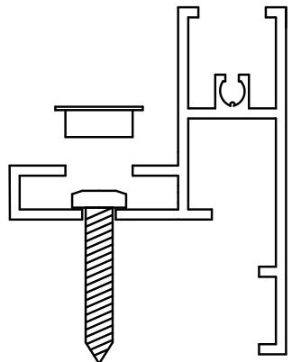
Secure the unit in place with a screw. Cover the screw hole with the cover cap supplied.
